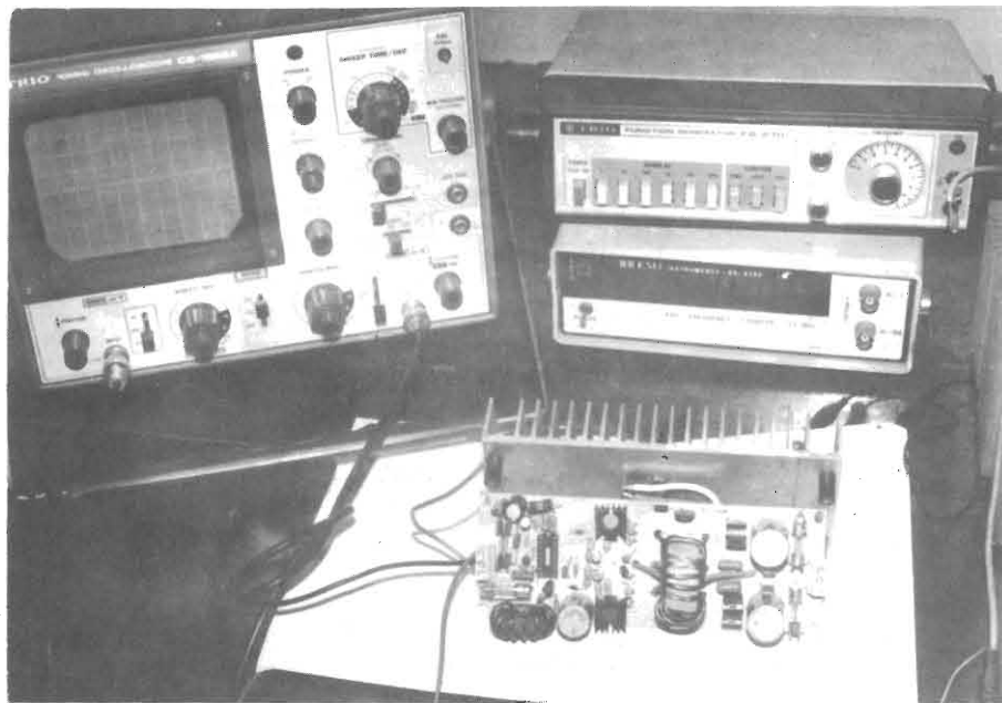
Inverter in prova
